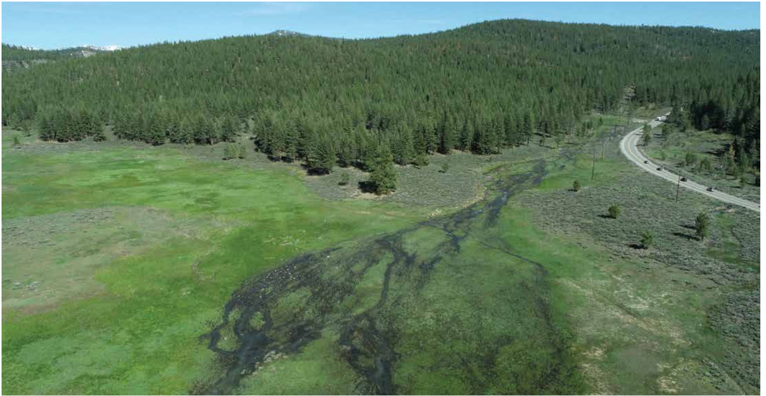
Martis Valley just north of Northstar. An altered channel was causing safety hazards from flooding on Rt.267 just north of Northstar. Now, the stream channel is restored to its original alignment, and replenishes the natural historic floodplain for a greener, wetter, wilder landscape. Photo: Balance Hydrologics, May 2023
